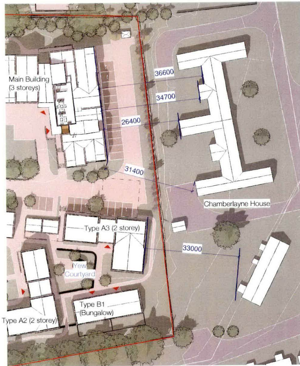
EXTRACT FROM PROPOSED SITE PLAN DRAWING 0103: Diagram showing minimum separation distances between facades
